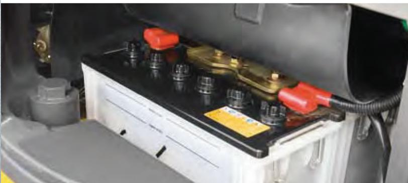
Dual 80 Amp Hr batteries are easy to access and protected by heavy-duty rubber cover.
