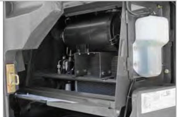
2-Stage engine air filter and radiator systems are accessible after removal of pre-filter screen.
