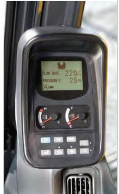
The Power Mode System provides four power modes to match your work operations. The monitor features a large sunshade and orange back-lit screen for easy daytime viewing.
